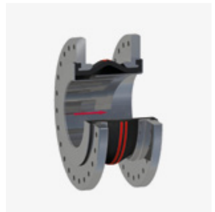
Telescopic inner sleeve (large axial movement absorption and full bellows protection)
