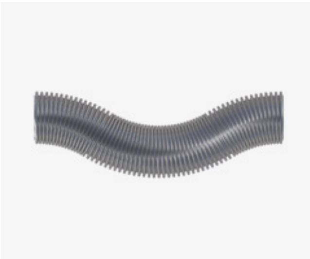
Column instability of a steel expansion joint
