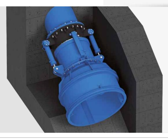
Narrow groove sliding penstock for fluids. Mechanically welded body, comprising two bolted parts, with internal guides for smooth movement of the penstock during operation and flat seat.
