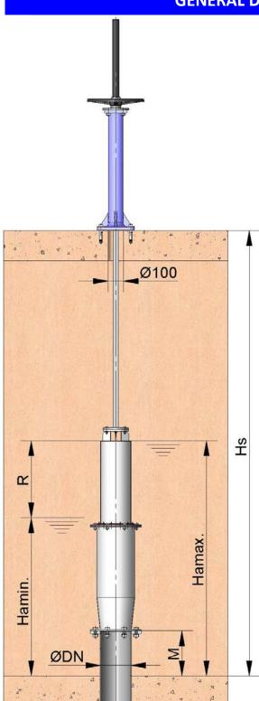
In order to define a **TE** telescopic valve, it is necessary to know the diameter of the run-off pipe, the flange bore standard and the required stroke. The stroke is defined as the difference between the upper and lower levels required.
