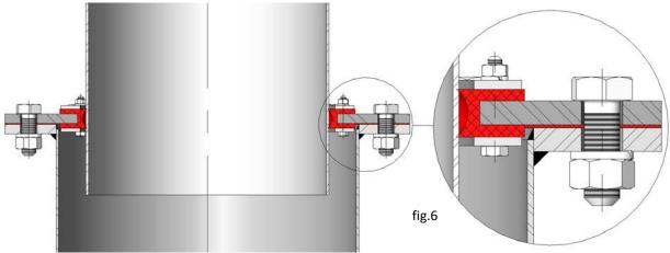
Although the standard seal is EPDM, there are other types of materials in order to choose the most suitable, in accordance with the working conditions of the valve (work temperature, fluid type, etc). The characteristics described below are the most common ones, and they are also summarised in table 2:
