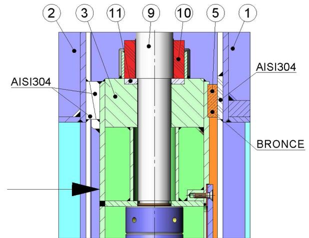
The only regular maintenance required for these penstocks is to change the gasket to carry out this task in the most straightforward way possible,
