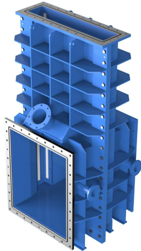
The clamping flanges of the penstock are usually rectangular, although circular ones can be produced to order. In any case, these flanges have a built-in elastomer seal, with the benefit of not requiring any additional seal between the conduct and the penstock.
