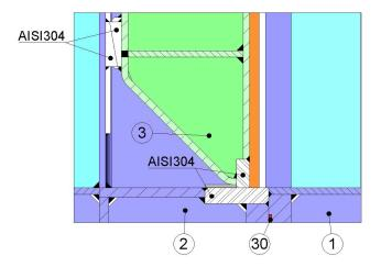
Since these penstocks are designed for use in water deposit run offs, the lower part of the penstock passage is completely smooth, thus preventing the build up of residue on the lower seal and ensuring there is no turbulence or cavitation.
