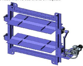
The blades are made flat, with reinforcing ribs and are supported on two semi-shafts. The flat blade system is sufficiently rigid for the working pressures of these valves and they do not produce significant load losses.
